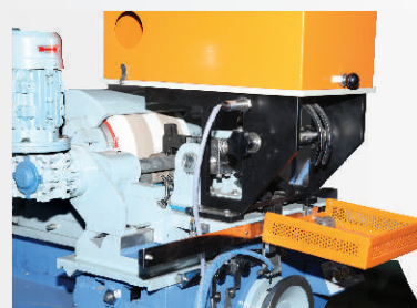
Automatic Grinding of Ring frame / Speed frame Top Rollers, Controlled by PLC-MMI. It is fitted with Auto feeding Box & Collecting basket.
